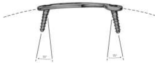
3 B The Standard Cranial and Caudal Angulation of Screws
